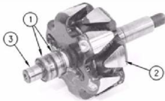
Gambar 4.37 – (1) Slip Ring, (2) Rotor, (3) Rotor Shaft
