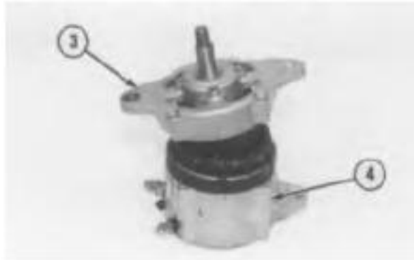
Gambar 4.15 memasang alternator housing
