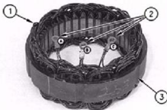
Gambar 4.40 – (1) Stator, (2) Stator Lead, (3) Stator Frame
