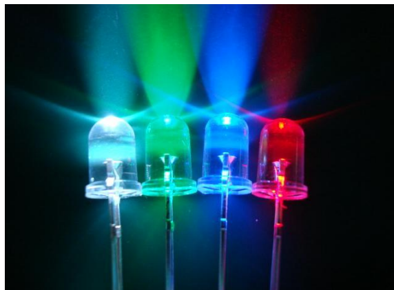
Gambar 3.5 LED Penghasil Macam-macam Warna
