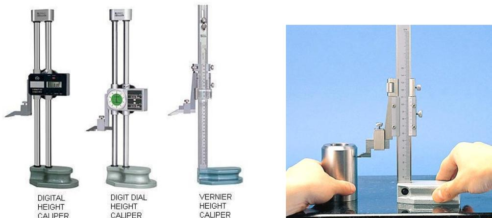
Gambar 7.7 Pengukur Tinggi (*Hight Gauge*)
