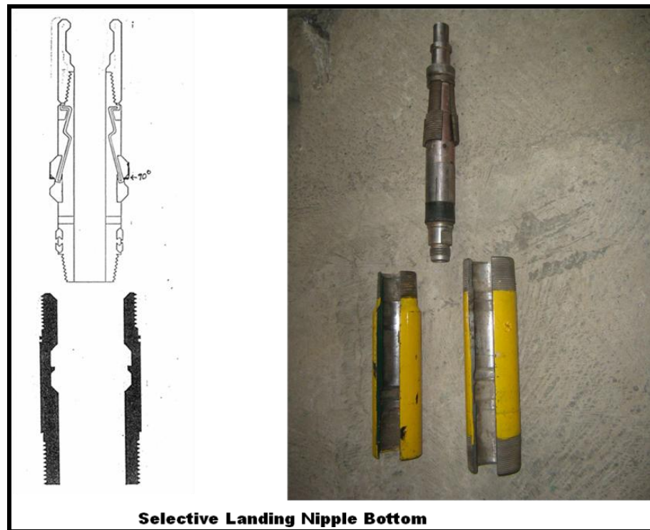
Gambar: 8 Selective Landing Nipple
