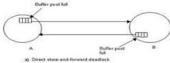
Gambar .13 Direct store and forward deadlock
