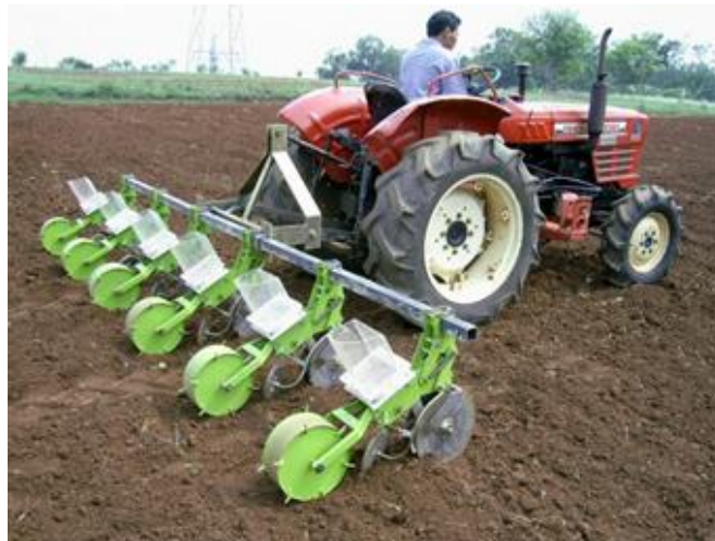
Gambar 58. Alat tanam sistem baris lebar
