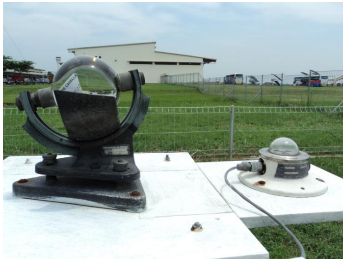
Gambar 85. Alat ukur lama penyinaran surya (Campbell stokes)
