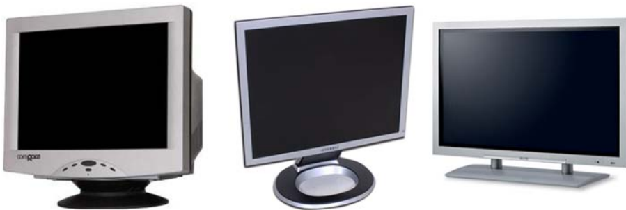
Gambar 3.25 Monitor (a) CRT; (b) LCD; (c) plasma
