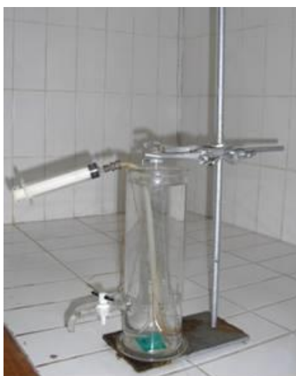
Figure 2 Equipment for extracting phosphine gas from an aluminum phosphide formulation (Busvine 1980).
