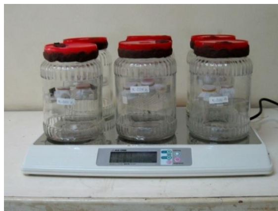
Figure 4 Magnetic stirrer for homogenizing phosphine gas distribution in the fumigation chamber
