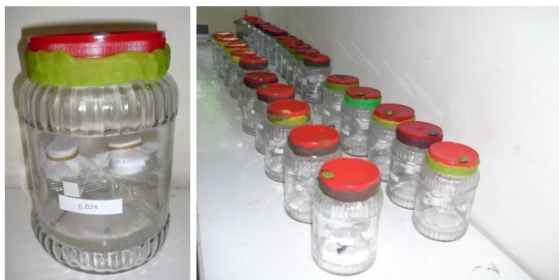
Figure 3 Glass jars as a fumigation chambers in phosphine resistance testing
