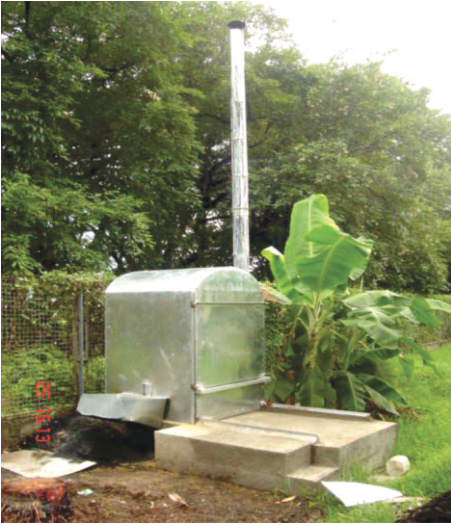
A cabinet type pasteurizer which is being fueled by rice hull (left photo) and recycled drums as pasteurizer (right photo).
